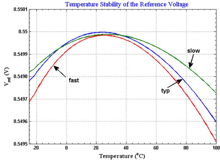
Figure 5: Variation of  $V_{ref}$  over different process corners
