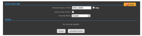
Network Name (SSID) — SSID (Service Set Identification) must be assigned to all wireless devices in your network. Considering your wireless network security.
