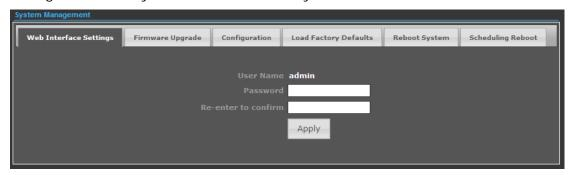
◆ Password — The new password must not exceed 32 characters in length and must not include any spaces. Enter the new password a second time to confirm it.
