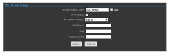
**802.1X WEP**: Selects WEP keys for data encryption. When enabled, WEP encryption keys are automatically generated by the RADIUS server and distributed to all connected clients. (Default: Disabled)
