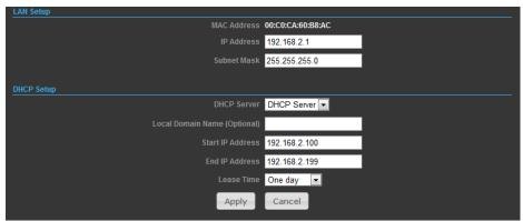
◆☐IP Address — The IP address of 2.4GHZ 802.11B/G/N AP/ROUTER on the local area network.
