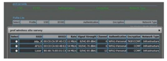
3) Now, it shows the Profile Name, SSID, BSSID, and encryption type received from your target network and press **Next** button to continue.
