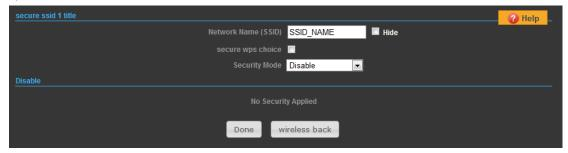
Network Name (SSID) — SSID (Service Set Identification) must be assigned to all wireless devices in your network. Considering your wireless network security.
