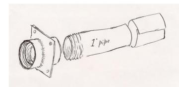
The air inlet is made from a 1" pipe nipple welded to a 1/8" plate. The air inlet is mounted 3" above the bottom of the reactor. Use RTV high temperature silicone to seal the flange to the container. Use #10 screws to bolt this plate to the reactor.
